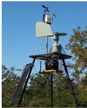
Figure 7: Mold spore, pollen and meteorological data collection station
